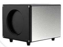
As a standard radiation source, black body has been widely used for calibrating infrared light system, measuring material emissivity, measuring parameters of infrared sensor, and transmitting temperature between infrared emitter and thermal device.
